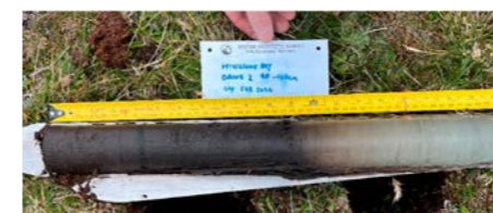
Peat core sample inside coring apparatus taken at Horseshoe Bay by BAS team, showing peat (brown, left) to clay (grey, right) interface.
