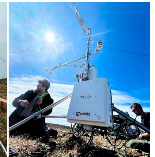
LEFT Ground anchor screws being installed to secure flux tower tripod against the typical high winds of the Falkland Islands; CENTRE Flux tower tripod with some units attached whilst survey work is carried out; RIGHT UKCEH team nearing completion of flux tower installation. Each tower took around three days to install.
