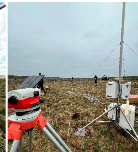
LEFT Ground anchor screws being installed to secure flux tower tripod against the typical high winds of the Falkland Islands; CENTRE Flux tower tripod with some units attached whilst survey work is carried out; RIGHT UKCEH team nearing completion of flux tower installation. Each tower took around three days to install.
