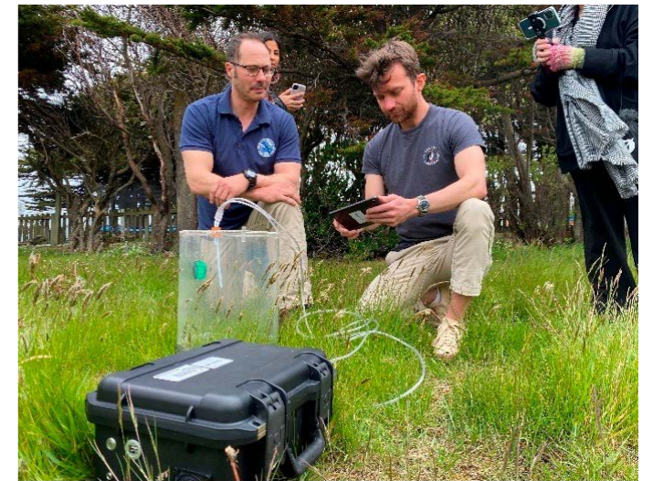
Falklands Conservation and SAERI demonstrating the use of a portable gas analyser (flux chamber) for the local media. The equipment will be used by the project.
