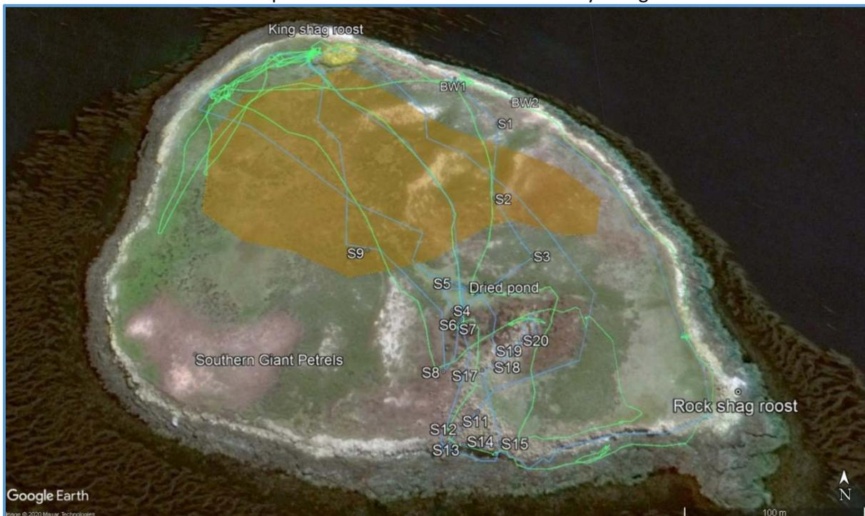
**Figure 19.** Ship Island survey features. Tracks show survey coverage. BW1 and BW2 show extents of boxwood planting. Bluegrass was planted around the dried pond. S1 through S20 show soil measurement points.
